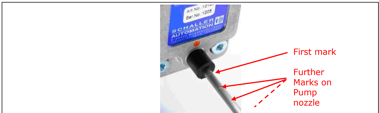
Figure 33: Marks on the nozzle
