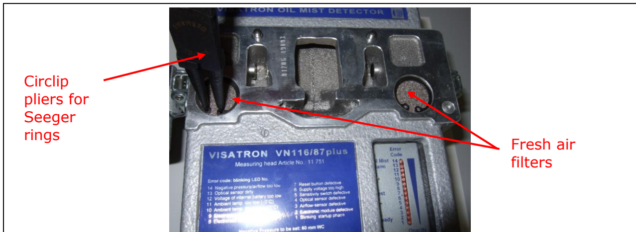
Figure 45: Exchange of the air filters
