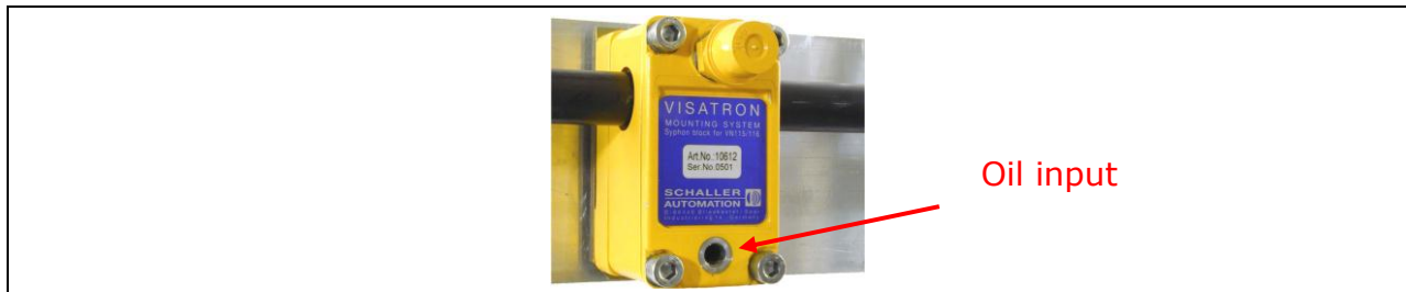
Figure 34: Siphon block VN180
