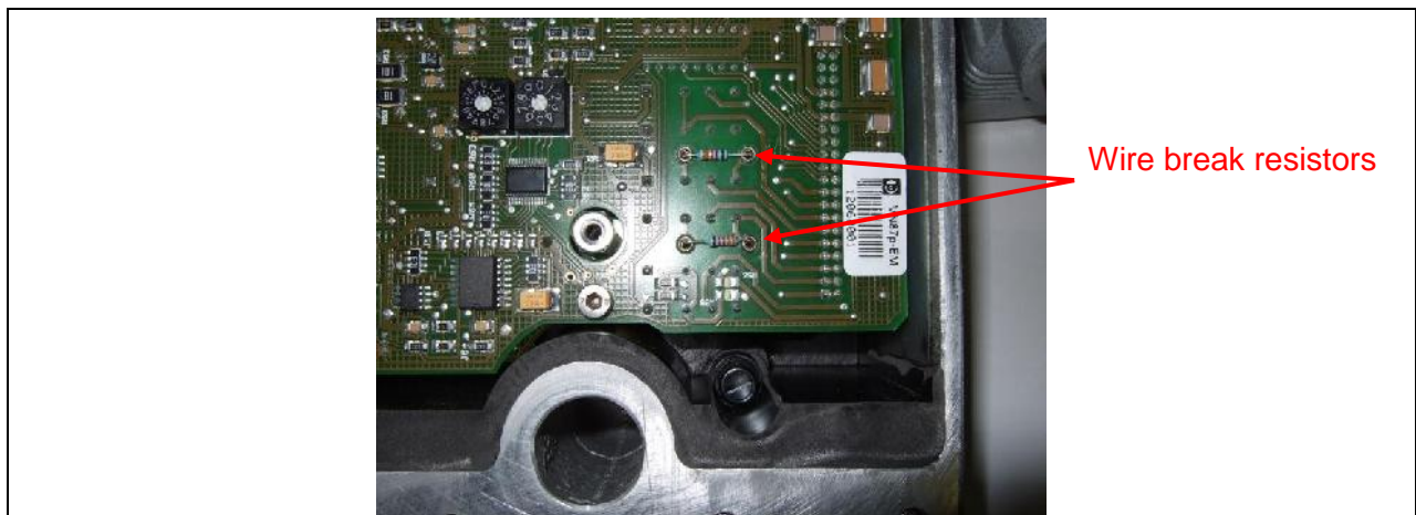
Figure 24: Wire break resistors
