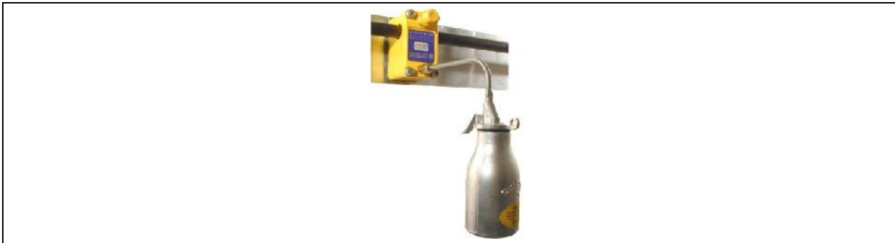
Figure 36: Filling pump inserted and fixed in the siphon block
