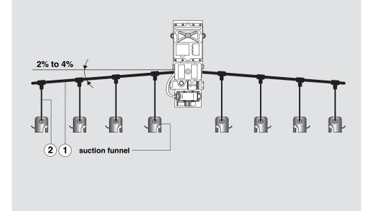
Consider to avoid oil collection when laying the headers! Oil must always drain back to engine
