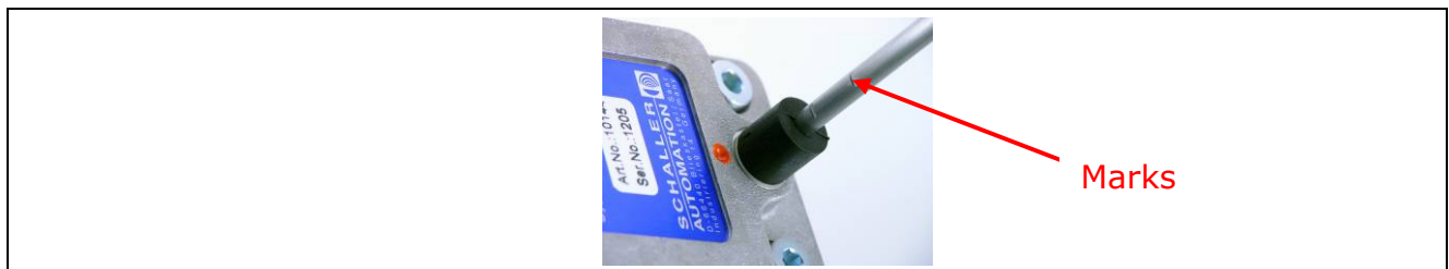
Figure 33: Marks on the nozzle
