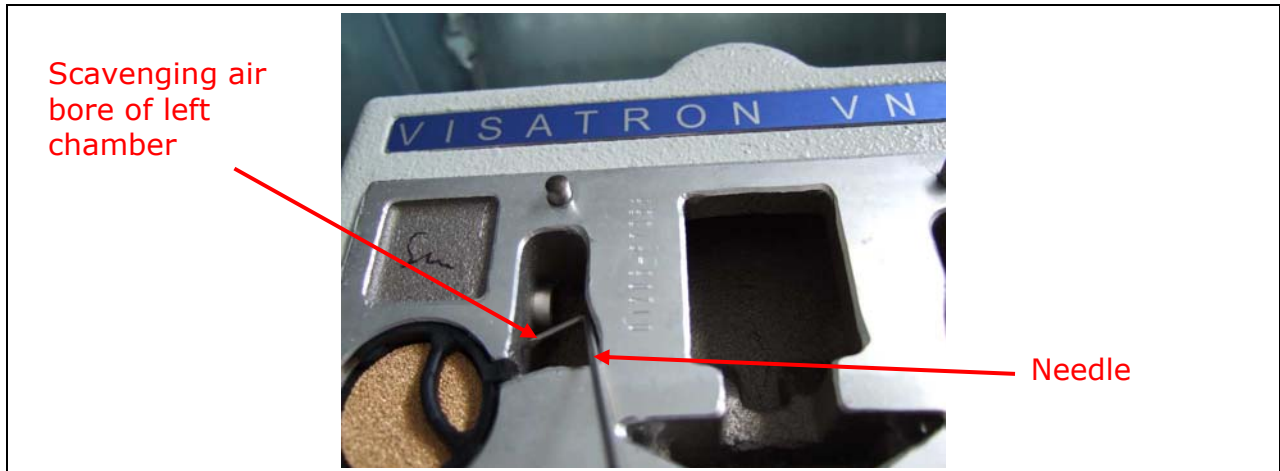
Figure 42: Cleaning of scavenging air bore in the left and the right chamber
