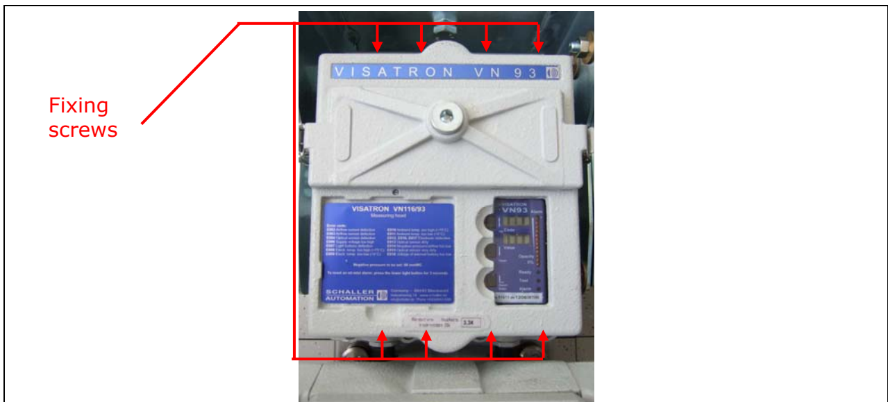
Figure 47: Step 2 is to unscrew the measuring head
